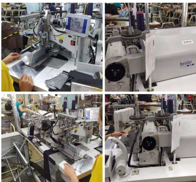
Photo Caption: Ionel SA equipped with high-end innovative Beisler sewing machine, for run stitching of straight and slanted openings, leading to productivity and competitiveness enhancement. Photo Credit: MCP
