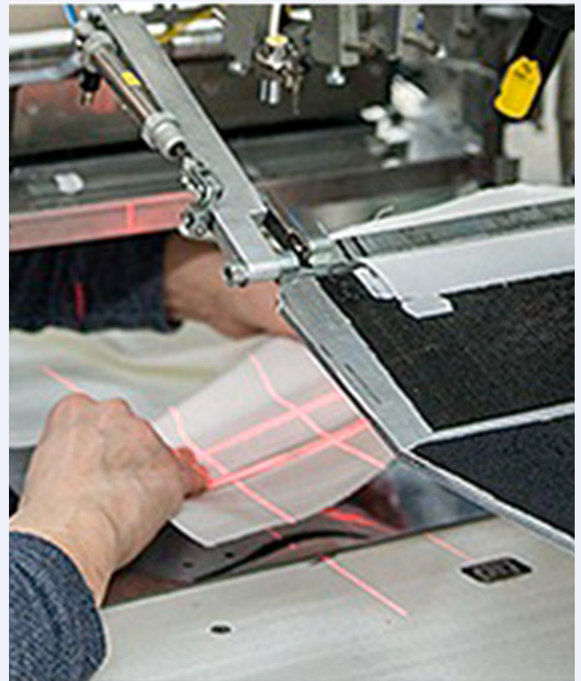
Photo Caption: Laser controlled for proper label positioning, proposed by MCP international consultant Martin Buecher. Photo Credit: MCP
